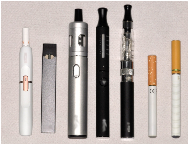
Figure 1. E-cigarette and heated tobacco devices in a range of designs. From right, two early devices that resemble a tobacco cigarette, so called 'cigalikes'; three 'tank' device which are refillable with e-liquids and rechargeable; a much smaller device that resembles an USB drive and uses nicotine salt technology; finally, a heated tobacco product with the tobacco stick in place.
